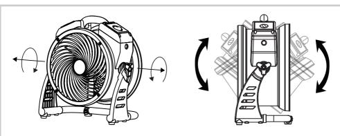
$\bullet$  The Air Circulator features 360  $^\circ$  Rotation. Tilt Air Circulator to desired angle and screw on rack handles to secure the position.
