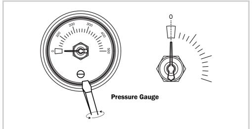
• Use a straight screwdriver to adjust the zero setting screw on the pressure gauge, until the pointer stays in the middle of the zero sector.
