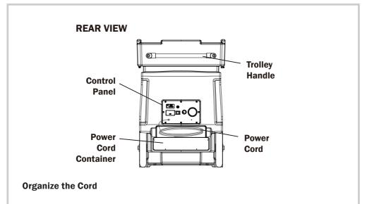
Power cord can be stored into the power cord container at the rear of the air scrubber.
